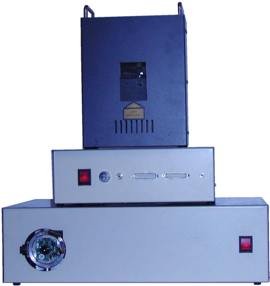
Figure D.1: The three encased experimental hardware units. The laser scanner, the control unit and the mechanical MAVE.
